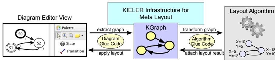
**Fig. 4.** Overview of the Kieler Infrastructure for Meta Layout (KIML).
